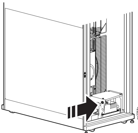
1. Position the leak sensor inside or outside the unit.
