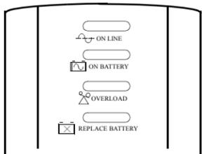
**On Line (green)** - is lit whenever utility power is powering the Battery Backup outlets.
