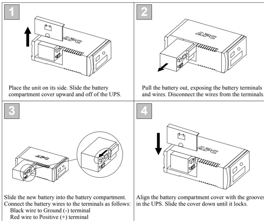
Place the unit on its side. Slide the battery compartment cover upward and off of the UPS.
