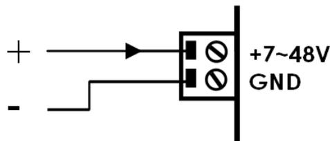
4. Reinsert the terminal block housing into the hubs casing. The "Power" LED on the hub should then light up green.
